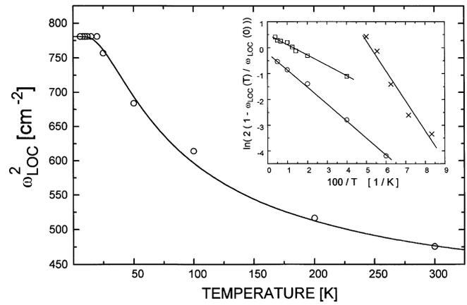
**Fig. 5.** Temperature dependence of the additional oscillator “strength” ( $\omega_{\text{LOC}}^2$ ). The solid line is calculated by (2). *Inset:* The  $\ln(2(1 - \omega_{\text{LOC}}^2(T)/\omega_{\text{LOC}}^2(0)))$  vs  $100/T$  dependence for  $\text{Pb}_{0.9}\text{Mn}_{0.1}\text{Te}(\text{In})$  –  $\circ$ ;  $\text{PbTe}(\text{G})$  –  $\square$ , and  $\text{Pb}_{0.75}\text{Sn}_{0.25}\text{Te}(\text{In})$  –  $\times$ . The solid lines are linear interpolations
