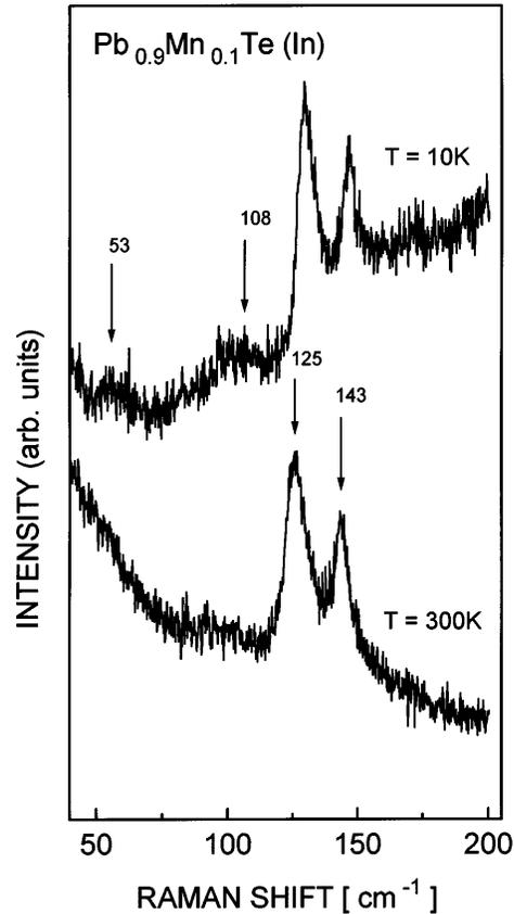
**Fig. 3.** Unpolarized Raman scattering spectra of  $\text{Pb}_{0.9}\text{Mn}_{0.1}\text{Te}(\text{In})$  measured at 300 at 10 K
