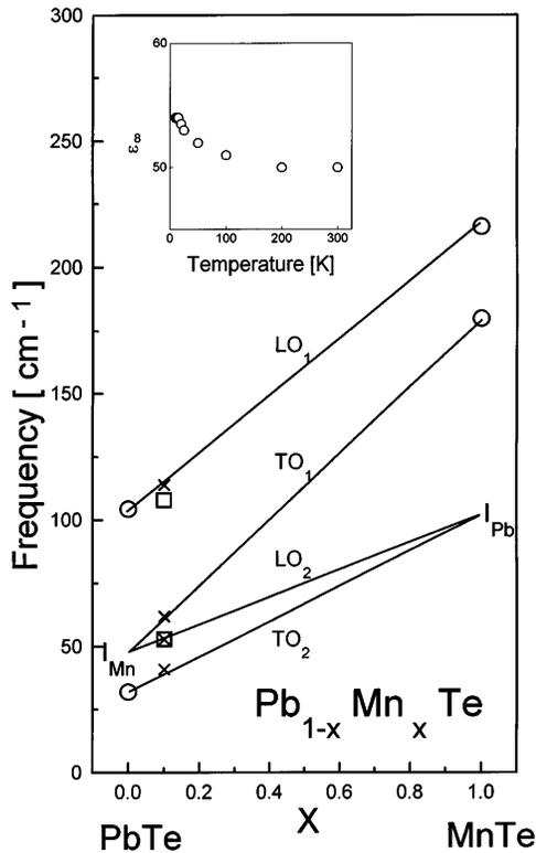
**Fig. 4.** Concentration dependence of the optical mode frequencies of  $\text{Pb}_{1-x}\text{Mn}_x\text{Te}(\text{In})$  single crystal.  $\times(\square)$  – IR (Raman) measurement of  $\text{Pb}_{0.9}\text{Mn}_{0.1}\text{Te}(\text{In})$ ;  $\circ$  – [17]. The solid line is a linear interpolation. *Inset:*  $\text{Pb}_{0.9}\text{Mn}_{0.1}\text{Te}(\text{In})$  high frequency dielectric constant ( $\epsilon_{\infty}$ ) vs temperature. The dashed line is a guide for eye
