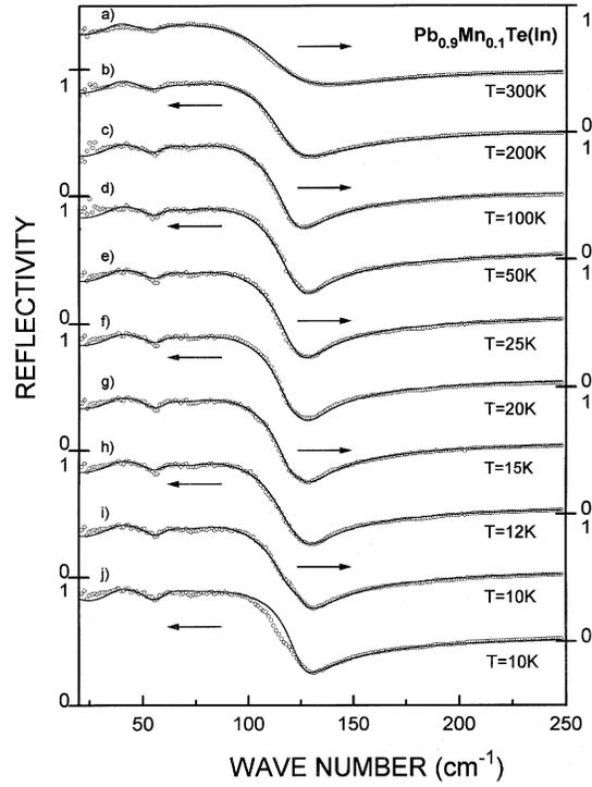
**Fig. 2.** Far-infrared reflectivity spectra of  $\text{Pb}_{0.9}\text{Mn}_{0.1}\text{Te}(\text{In})$  single crystal measured at different temperatures. The experimental spectra are represented by circles. The solid lines are calculated spectra obtained by using fitting procedure based on the model given by (1). All the parameter values have been given in Table 1. For  $T = 10$  K, the calculated spectra are given with (i) and without (j) additional oscillator at  $122$   $\text{cm}^{-1}$
