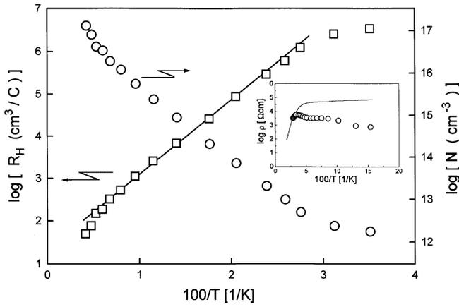
**Fig. 1.** Temperature dependence of the  $\text{Pb}_{0.9}\text{Mn}_{0.1}\text{Te}(\text{In})$  Hall coefficient ( $R_H$ ) and free carrier concentration ( $N$ ). *Inset:* Change of specific electrical resistivity vs. temperature for the unilluminated (solid line) and illuminated (open circles)  $\text{Pb}_{0.9}\text{Mn}_{0.1}\text{Te}(\text{In})$  single-crystal sample
