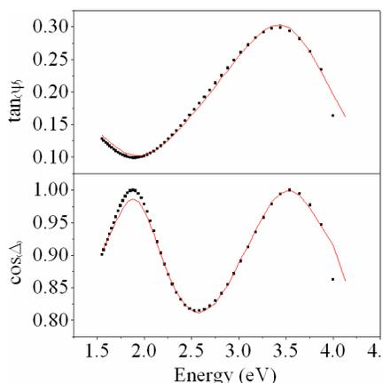
Measured ellipsometric parameters (circles) of thin films on a glass substrate and the best fit (full line)
