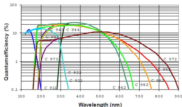
Fig. 15. Photon Counting Module MP 983, with spectral sensitivity –curve C983.
