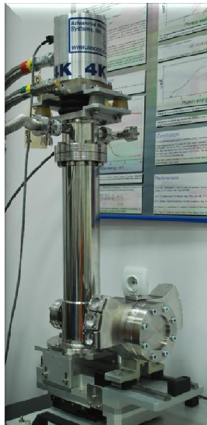
ARS DX204 closed cycle cryostat with SOPRA vacuum shroud.
