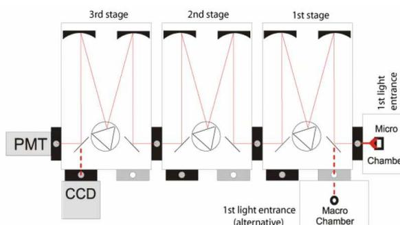
Fig.9. Triple Raman Spectrometer in additive or subtractive mode with Macro- or Micro-Chamber and PTM and CCD detectors.
