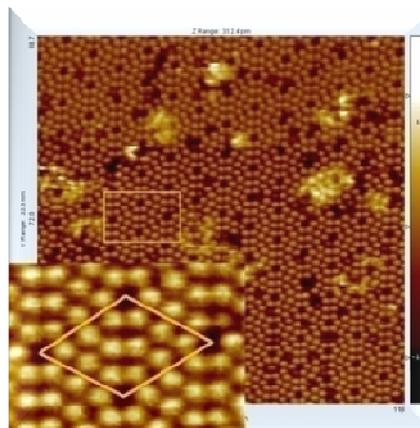
*Atomically resolved 7x7 reconstruction Si(111) (new surface atom rearrangement obtained by heating the sample to high temperatures under UHV conditions), STM mode.*
