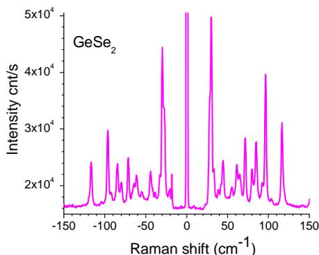
Fig. 12 Stokes and Anti-Stokes Raman spectra of GeSe<sub>2</sub>
