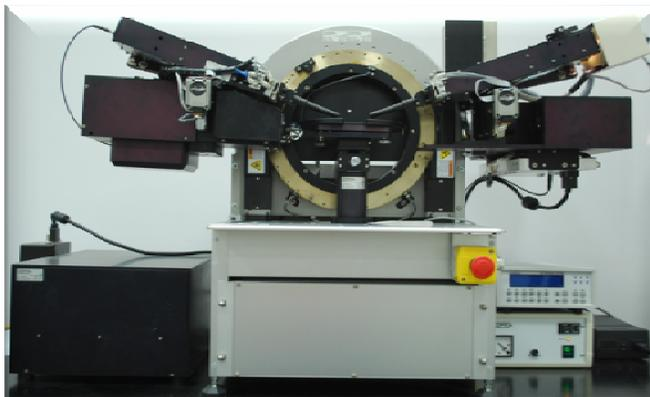
*GES5E-IRSE Spectroscopic Ellipsometer*
