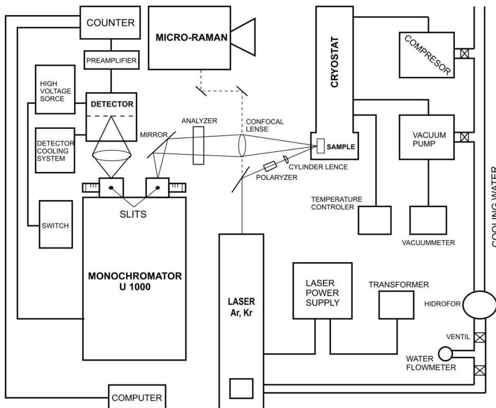
Detailed scheme of the Raman scattering and photoluminescence experiment.
