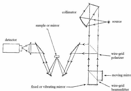
Configuration of SPECAC 40000 spectrometer for reflectance measurements
