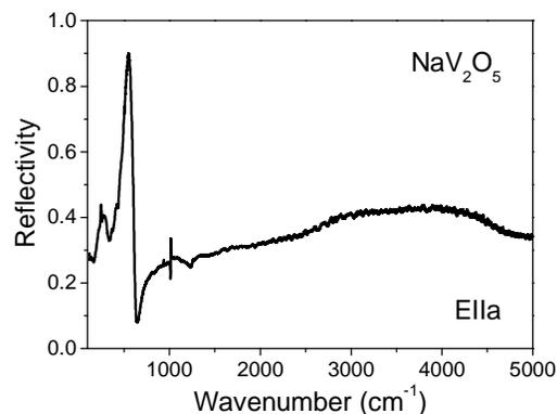
Fig. 4.  $E||a$  polarized FIR and MIR reflectivity spectrum of  $\text{NaV}_2\text{O}_5$
