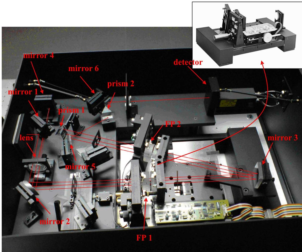
Figure 14. Brillouin JRS Scientific spectrometer. Inset: Tandem Fabry Perot interferometer with a common scanning stage
