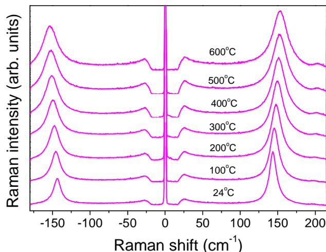
Stokes and anti-Stokes Raman spectra of  $\text{TiO}_2$  measured using Linkam stage in the 24 – 600 °C temperature range.
