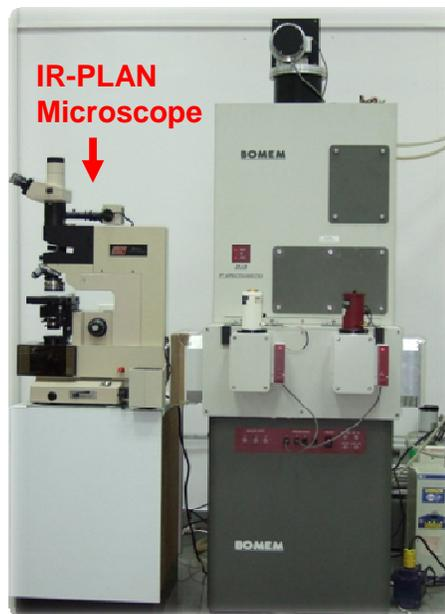
*Fig. 1. The Bomem DA8 spectrometer (to the right) with the InSb and Si detectors and Spectra-Tech IR-PLAN advanced analytical microscope mounted to the left port.*
