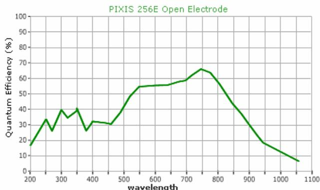
Fig.11. Quantum efficiency of Spec-10: 256E
