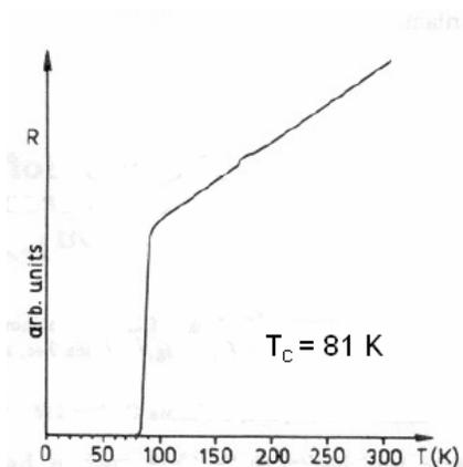
*Electrical resistivity of  $YBa_2Cu_3O_7$  superconducting oxide.*
