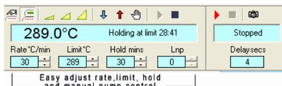
*The Linksys 32 software displays the live temperature, active ramp information and allows for the user to have full control of the rate of heating, limit and hold time*
