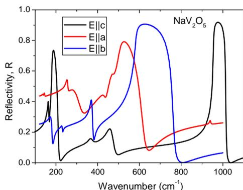
Fig. 3. Polarized FIR reflectivity spectra of  $\text{NaV}_2\text{O}_5$
