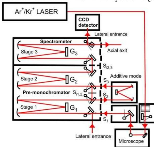
Fig.7. Optical diagram of JY T64000 monochromator in a triple additive and subtractive mode.
