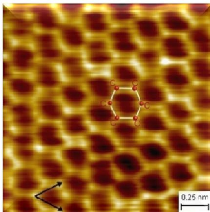
*Highly oriented pyrolytic graphite (HOPG), atomically resolved, AFM contact mode.*
