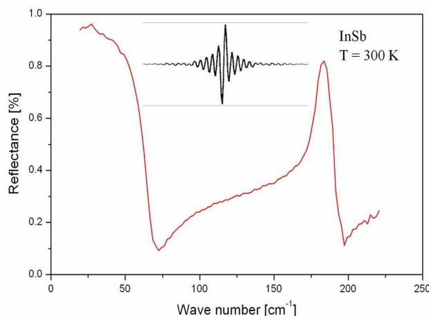
Fig.5. FIR reflectivity spectrum of InSb measured using Specac system at 300 K
