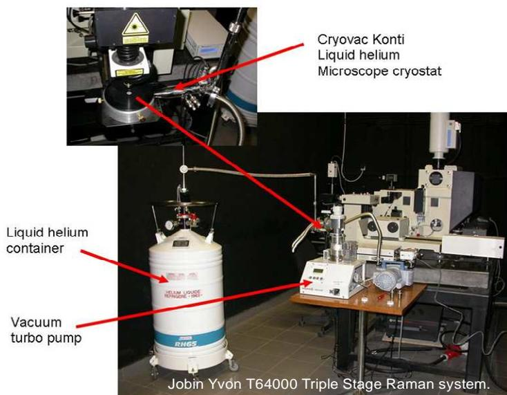
Jobin Yvon T64000 Raman scattering system with Cryovac Konti microscope cryostat.
