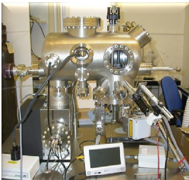
*Omicron UHV VT AFM/STM Microscope*
