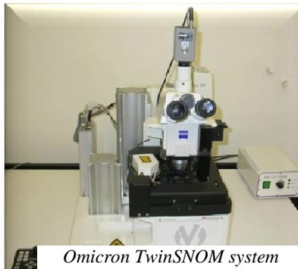
The SNOM fiber tip and the shear-force detector are integrated into a single magnetically mounted and easily exchangeable sensor module. A precise positioning is provided by the use of piezoelectric stepper motors. These motors are used for the remote controlled positioning of the microscope table as well as for the precise positioning of the sensor unit at the focus of the objective. The scanner unit is integrated into the microscope table.
