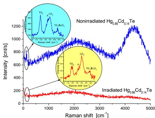
Raman (insets) and photoluminescence spectra of  $Hg_{0.86}Cd_{0.14}Te$  single crystal
