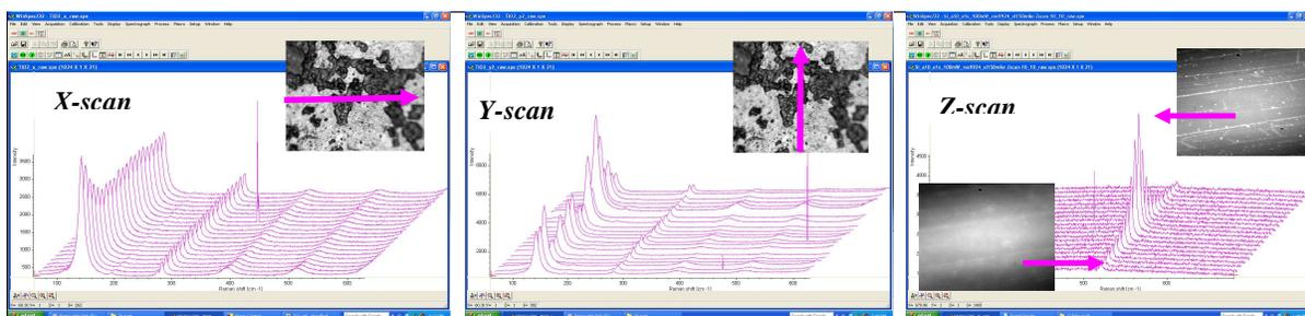
*X-scan and Y-scan: Raman spectra of the TiO<sub>2</sub> at various positions on the sample along x-and y-axes
