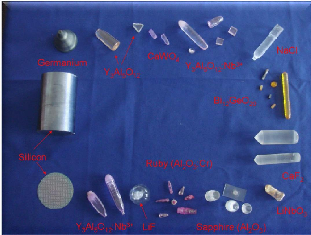
Single crystals of several semiconductors and optical materials obtained in our laboratory using the Czochralski, Bridgman and floating zone techniques.
