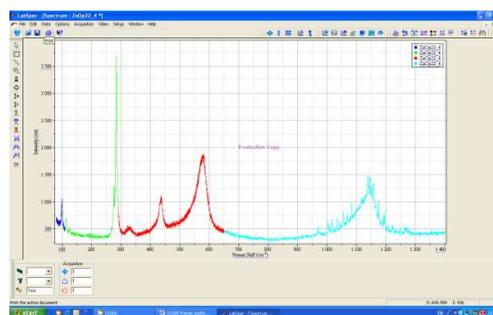
Figure 6. Raman spectrum of mechanically activated ZnO powder.
