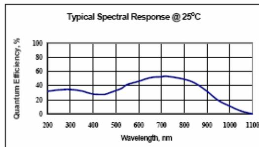
Fig.8. Quantum efficiency of CCD detector.
