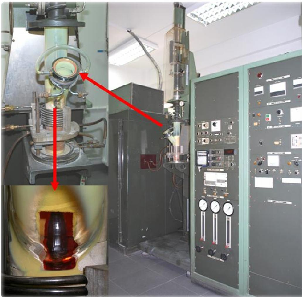
Czochralski crystal growth system (Metals Research Co). Crystal ingot is  $Bi_{12}GeO_{20}$ .
