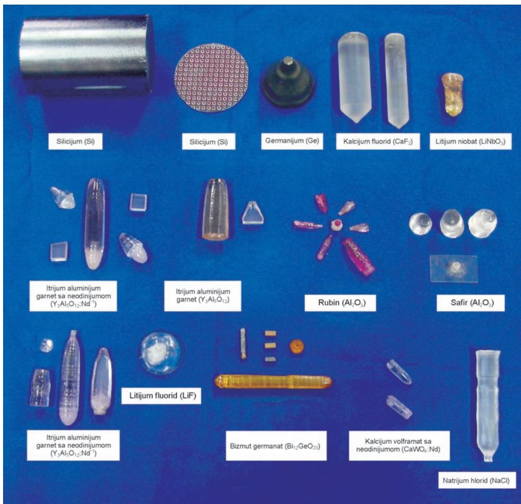
Single crystals of several semiconductors and optical materials obtained in our laboratory using the Czochralski, Bridgeman and floating zone techniques.
